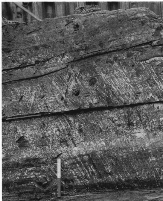
101. Billingsgate Lorry Park: a sawn plank from the 13th-century BG14 revetment. The diagonal saw marks preserved on the reverse face diverge either side of the 2 x 100mm scale, leaving the triangular signature characteristic of timber sawn on a single trestle, by the 'see-saw' method.
