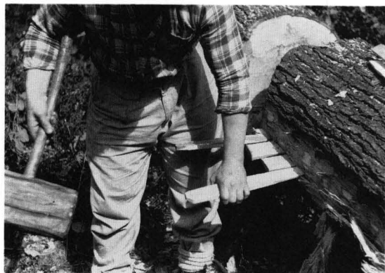
99. Converting timber using Saxon methods: cleaving halved timbers from a medium-sized oak standard with hardwood wedges.
